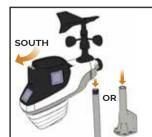
2 Remove rain gauge stabilizer from outdoor device.
